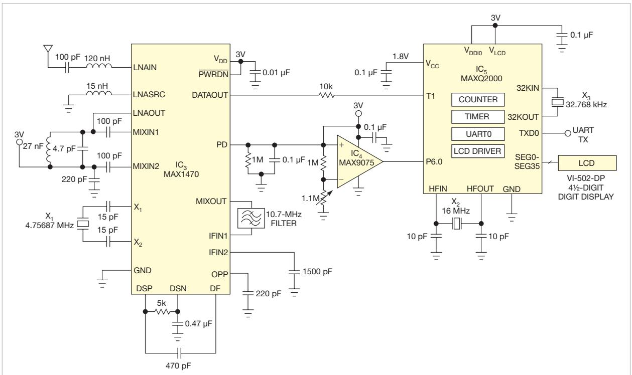
Figure 2 An ASK receiver with a microcontroller processes and displays temperature data.
